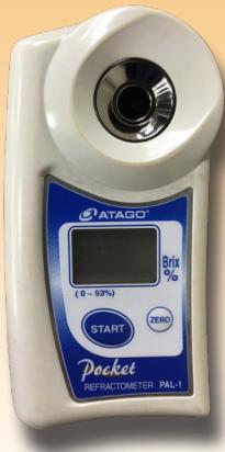
Since refractometer readings are temperature dependent, the measurement is only valid for the temperature of the liquid as it is being measured. Once any variable—water, concentrate/sub batch, or temperature—is changed, the brix reading is no longer a valid one.
