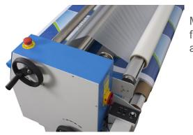
Motorized rear rewind for roll-to-roll applications
