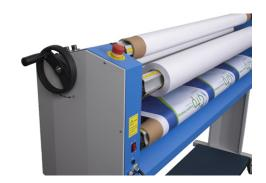
Integrated Rear Rewind makes Roll-to-Roll applications easy.
