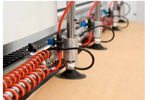
The suction grippers shake and bend the sheet to separate the material.
