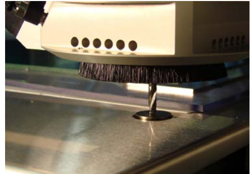
The automatic knife tip sensor regularly checks knife blades and milling bits.
